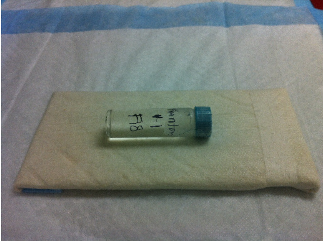
Figure 43: Radionuclide filled vial, containing 16.8 mL of water. This vial serves as a phantom for sensitivity and count rate linearity measurements for ^{52}\text{Mn} , ^{18}\text{F} , and ^{89}\text{Zr} .
