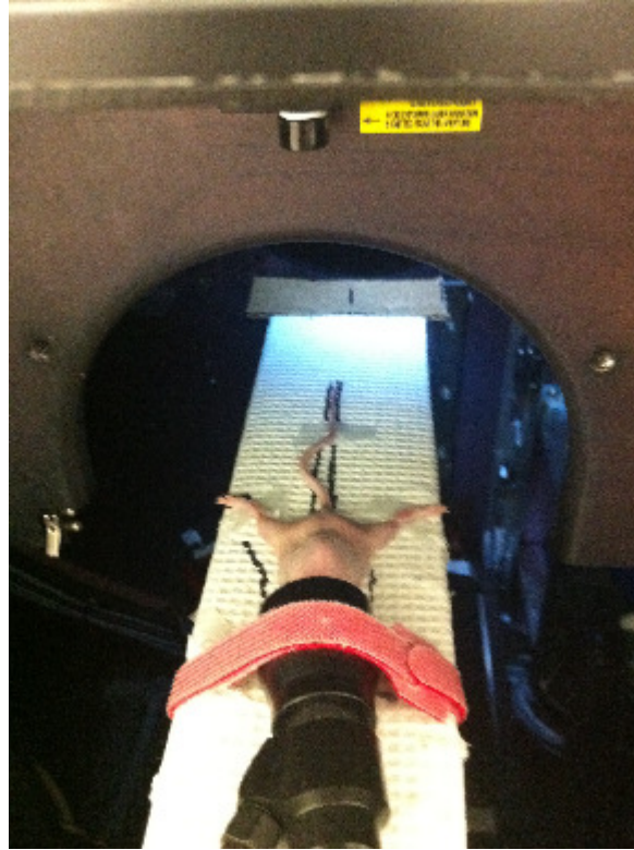
Figure 54: Each mouse in the imaging study had an individualized pallet that was used in both the MR and PET scanners. An outline of the mouse was drawn to increase positioning reproducibility, but because of the different shaped nose cones of the scanners, positioning was not entirely reproduced.
