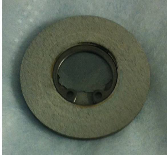
Figure 7: The target assembly used to support the chromium in the cyclotron beam. The chromium foil target (center) is held to the iridium holder (outside) by a steel clip (middle) during the irradiation.
